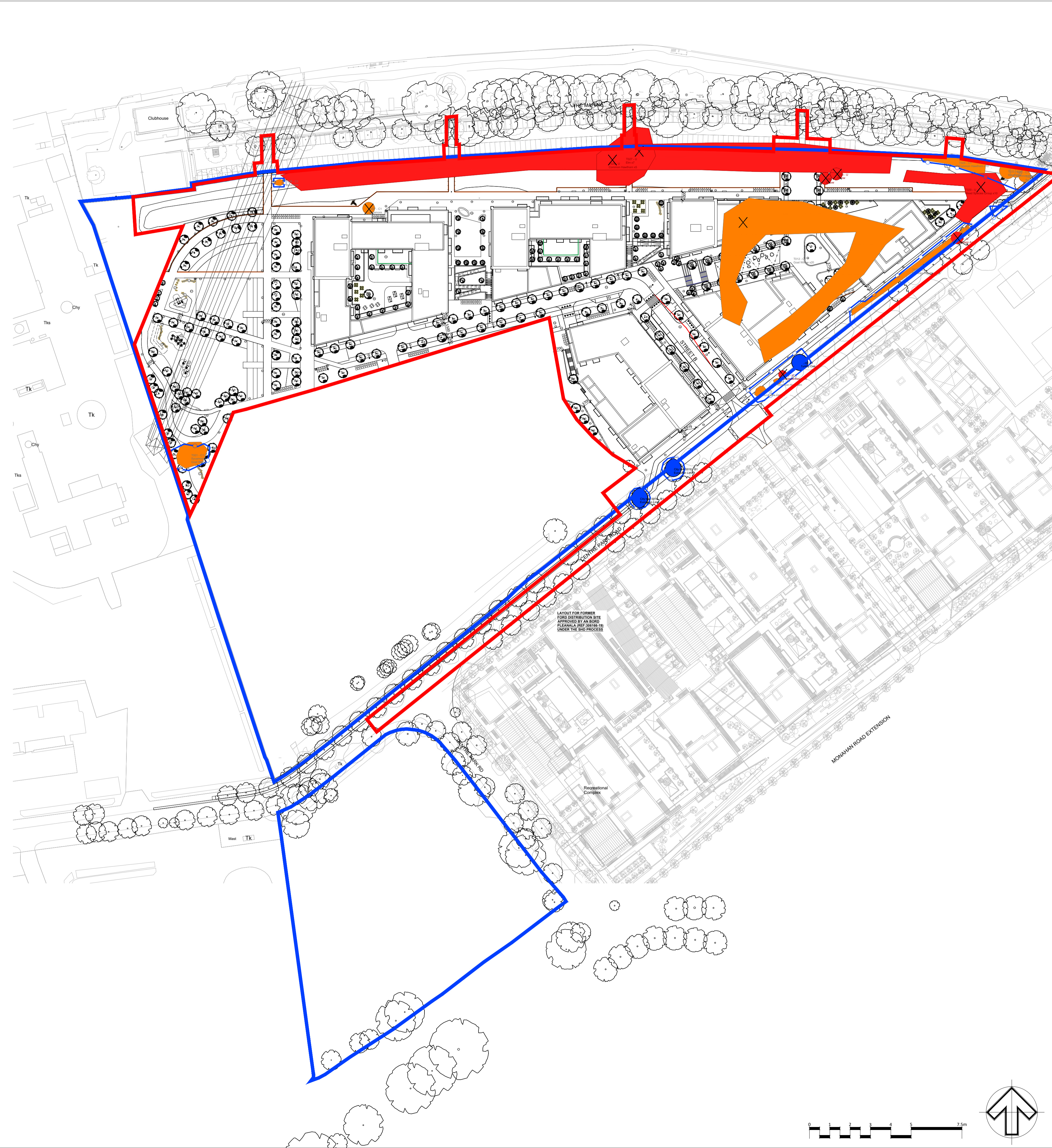
FIGURE1: Tree Protection Fences based on Figures 2 and 3 as per BS 5837:2012
